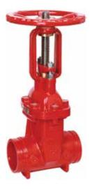
Size : 2", 2<sup>1</sup>/<sub>2</sub>", 3", 4", 5", 6", 8", 10", 12" Working Pressure : 20,7 bar (300psi) Max. Test Pressure : 41,4 bar (600psi) **Working Temperature** :0-80°C Connection : Grooved metric or AWWA C606 standard **Specifications** : Design and dimensions conform to AWWA C515 : Fusion bonded epoxy coating in **Corrosion Protection** accordance with ANSI/AWWA C550 for both interior and exterior surface. Features : Pre-notched, stainless steel stem for easy
