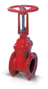
Size : 2", 2<sup>1</sup>/<sub>2</sub>", 3", 4", 5", 6", 8", 10", 12" Working Pressure : 20,7 bar (300psi) Max. Test Pressure : 41,4 bar (600psi) :0-80°C Working Temperature Connection : Flange diameter and thickness according to ANSI B16.1 Class 125, EN1092-2 PN10 or EN1092-2 PN16 **Specifications** : Design and dimensions conform to AWWA C515 **Corrosion Protection** : Fusion bonded epoxy coating in accordance with ANSI/AWWA C550 for both interior and exterior surface. Features
