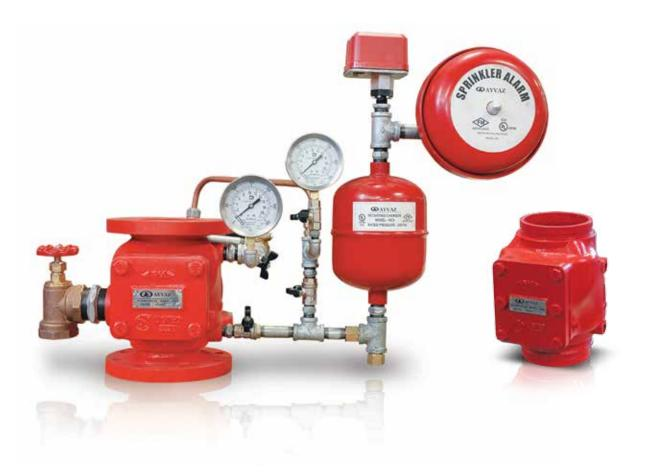
Size: 3", 4", 6" & 8"Max. Working Pressure: 17.5 bar (250 PSI)\*Mounting: VerticalFlange Connection: ANSI B16.42 #150Trim: GalvanisedCoating: Red PaintFactory Hydrostatic: 35 bar (500PSI)
