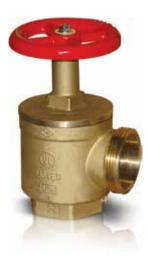
Sizes available (Nominal): DN40/11/2", DN65/21/2"Working pressure: 20.6 bar (300 psi)Finish: Polished Brass and Polished ChromeConnections: Female threaded NPT inlet and male<br/>threaded NST outletSpecifications: Used with fire hoserack assembly or fire<br/>department outlet connection
