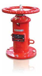
Wall indicator post provides a means to operate a valve installed behind a wall and able to indicate the open or shut position of the valve.
